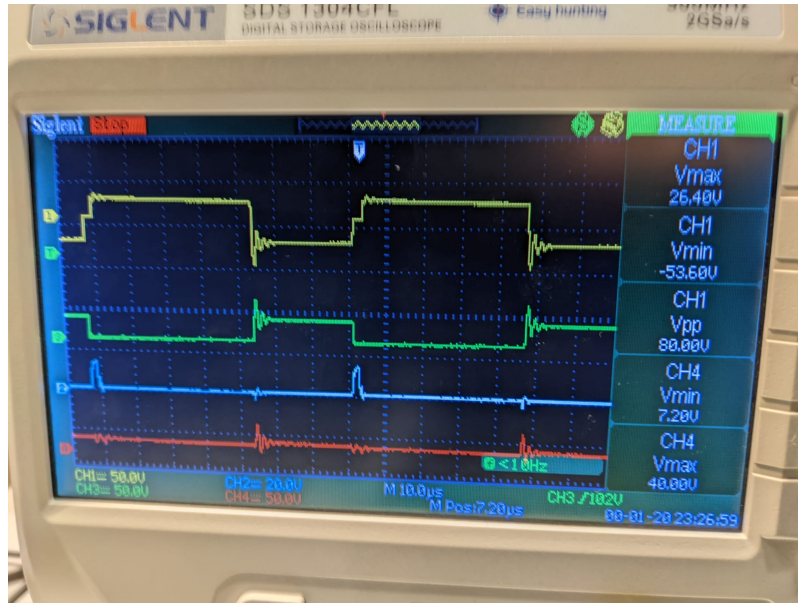
Transformer voltage, Q3, Q2, battery voltage, from top to bottom
