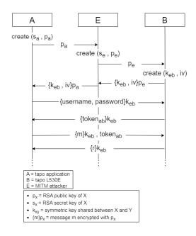
Fig. 8. Sequence chart for the attacker's MITM between app and bulb
