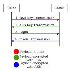
Fig. 6. Tapo Symmetric Key Exchange Protocol
