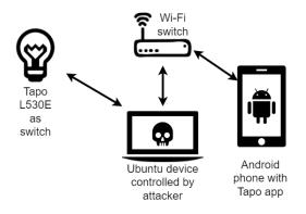
Fig. 4. Setup C, network with a non-configured bulb
