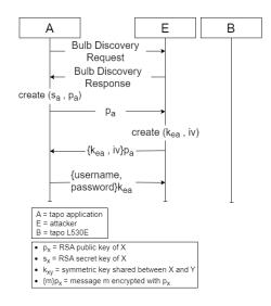
Fig. 7. Sequence chart for the attacker's impersonation of the bulb
