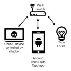
Fig. 3. Setup B, network with a configured smart bulb
