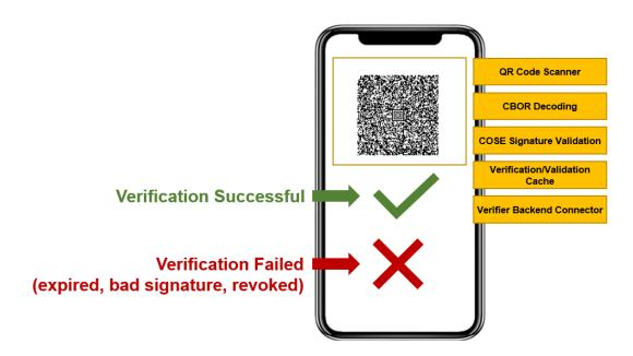
Figure 13: Core components of the verifier app
