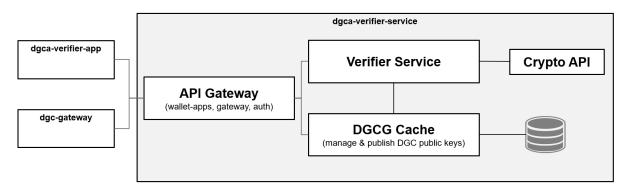
Figure 14: Verifier application backend building blocks
