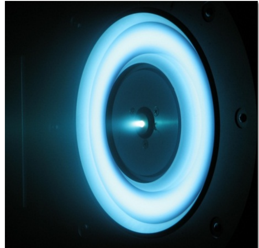
NASA's 3000-s Isp, Magnetically-shielded Hall Thruster
