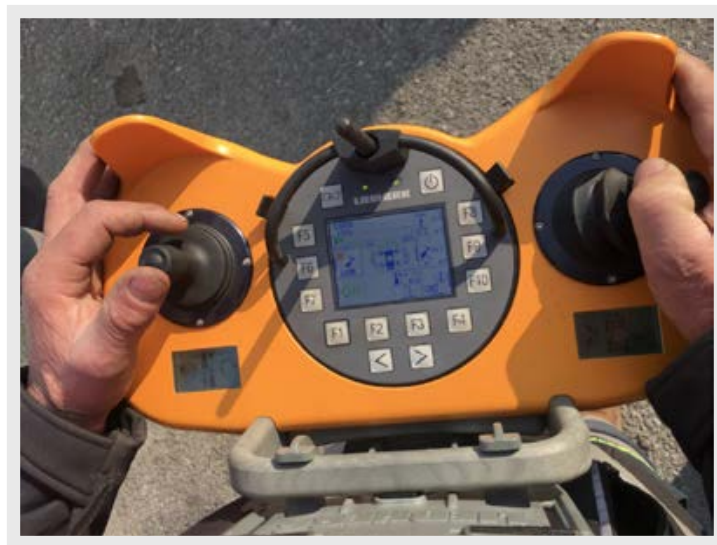
Figure 51. Liebherr industrial radio remote controller, which we found at a transportation business, using standard Bluetooth
