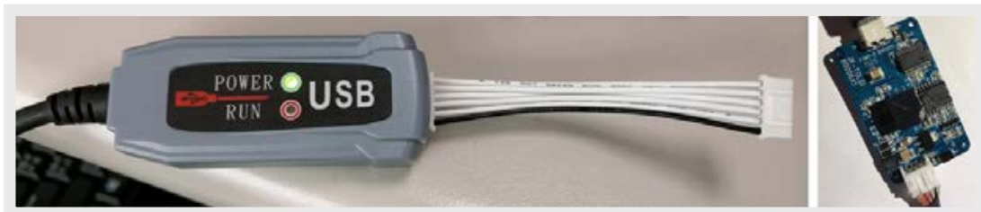
Figure 19. Saga and Juuko (opened) programming dongles. Telecrane uses the same programming dongle as Saga.
