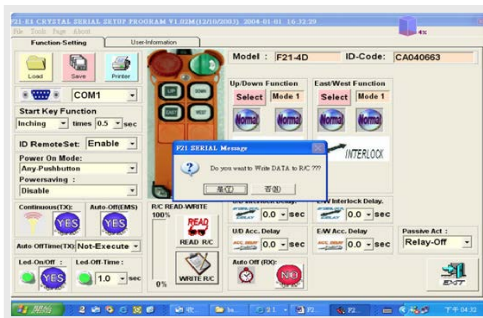
Figure 42. Screenshot obtained from the Telecrane programming manual, not mentioning any authentication steps 64
