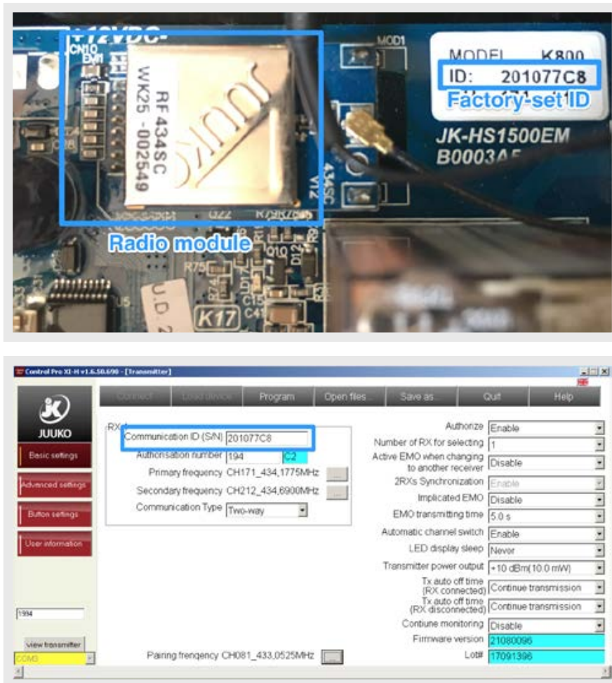
Figure 8. ID printed on the enclosure of a unit that we analyzed and on the programming software that allows the user to change it (consistently on TX and RX)
