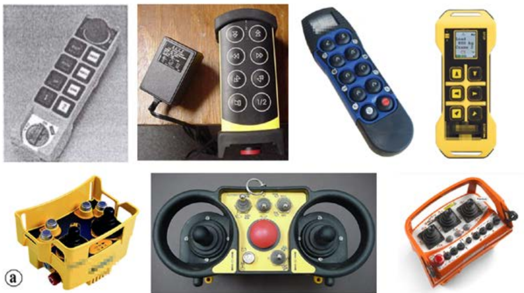
Figure 1. Evolution of hand-held and belt-pack remote controllers (main steps from 1997 to 2018), as seen in photos from user manuals and FCC documentation
