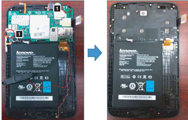
Figure 5. Removal steps of system board
