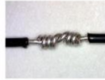
Figure 19-17. Completed Wrap for Western Union/Lineman Splice
