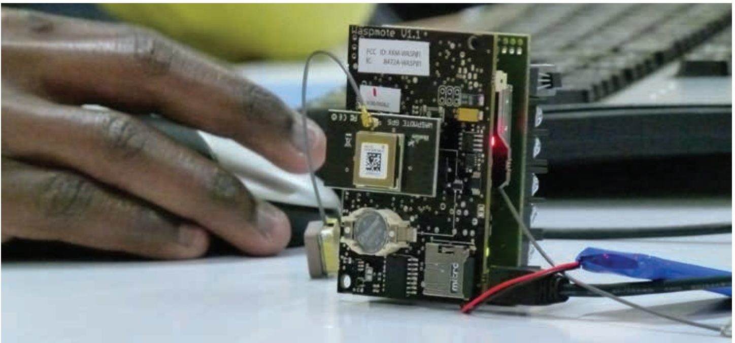
Photo credit: Marco Zennaro. GSM connectivity node in Nairobi.
