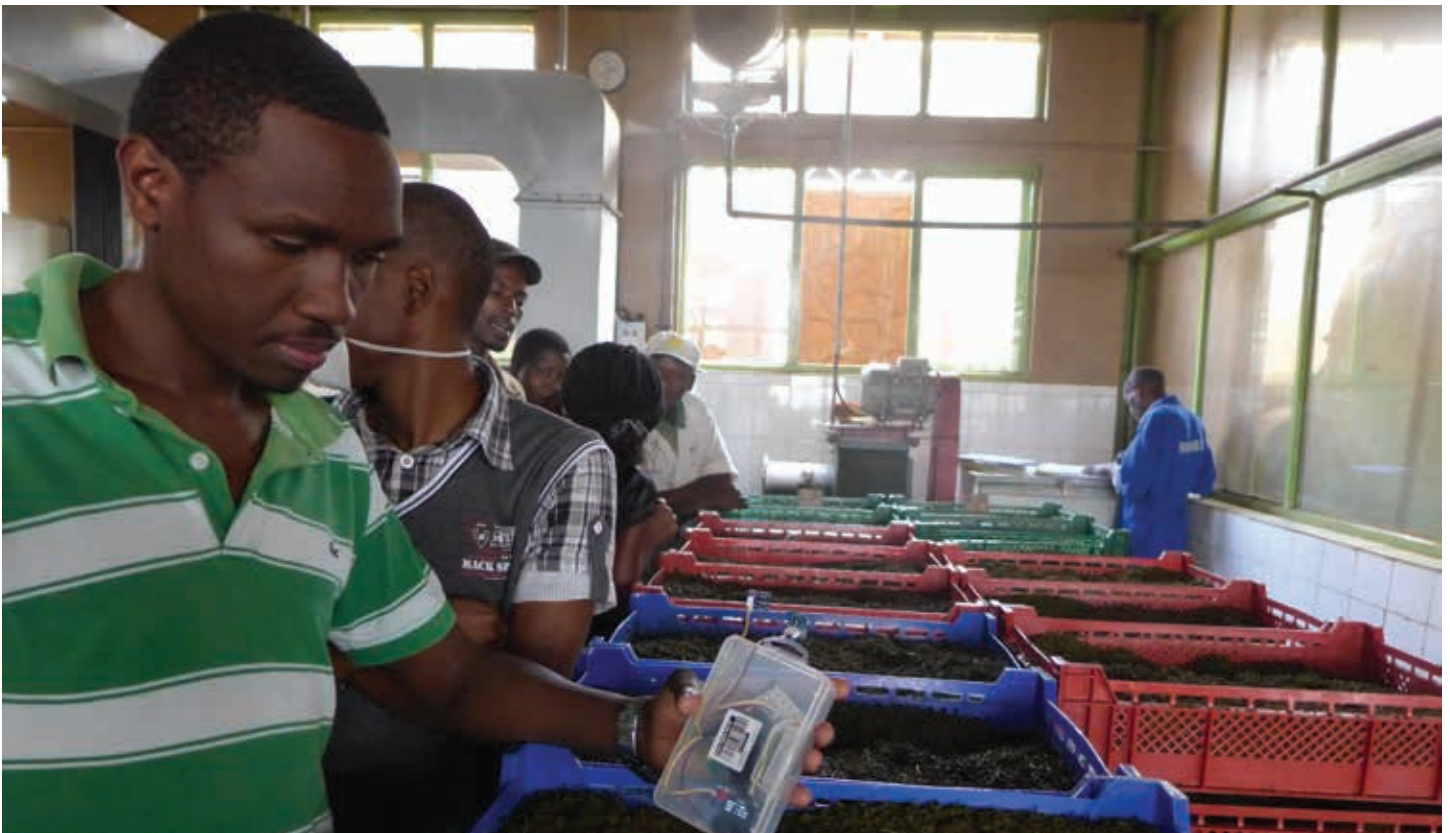
Photo credit: Marco Zennaro. Engineer with a GSM-enabled soil moisture sensor node in a tea factory plantation in Rwanda.
